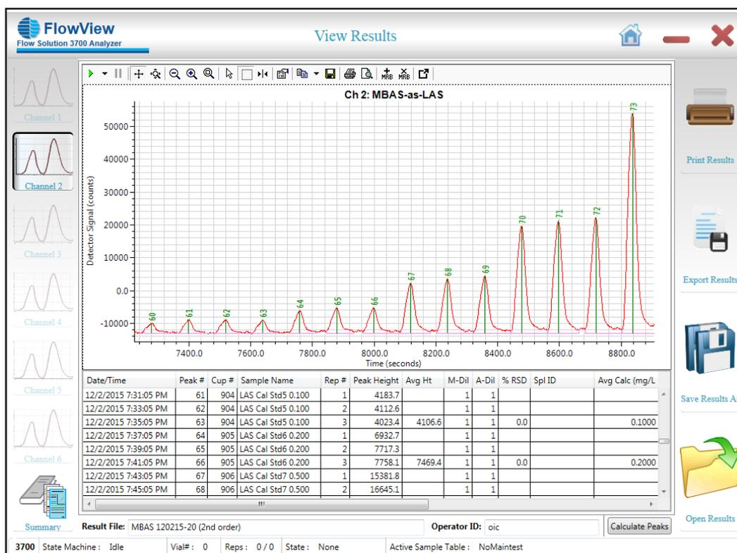
Figure 2. MBAS Calibration Series
